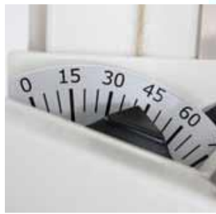
Indication of the transversal arm rotation angle
